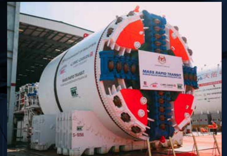
THE MACHINE: The cutting wheel of the Variable Density Tunnel Boring Machine - the front end of the 135m-long machine that will bore through surfaces for the construction of the underground tunnels for the SSP Line.
