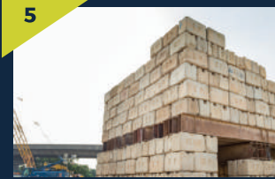
Kentledge blocks for the Maintained Load Test (MLT) at the Kepong Sentral Station site.
